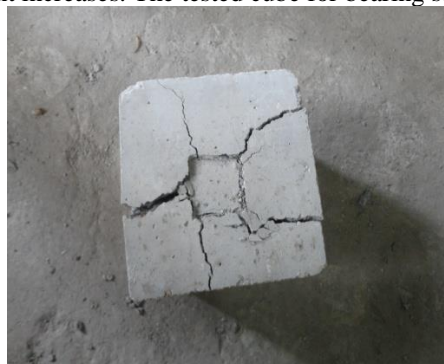
Fig.2: Tested cube (bearing test)
